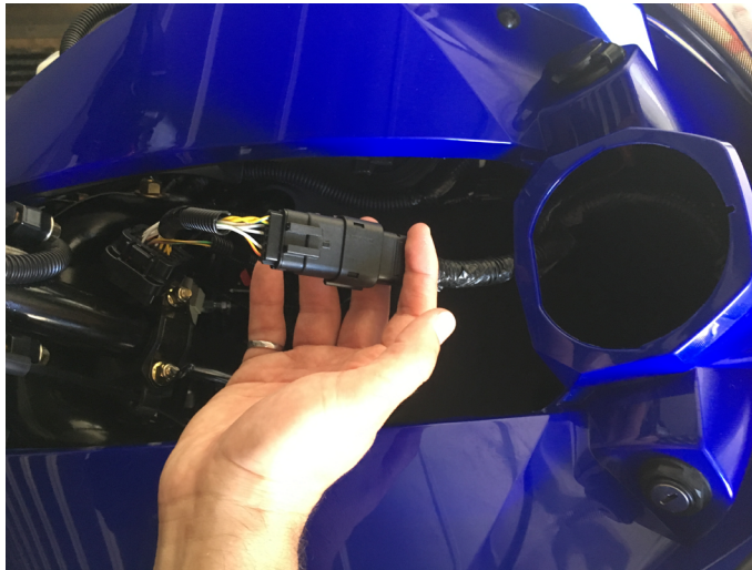
Figure 28. Connection of the Anti-Lag cable harnesses and instrument cluster
