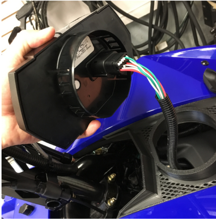
Figure 23. Instrument pack connection to the Anti-Lag harness
