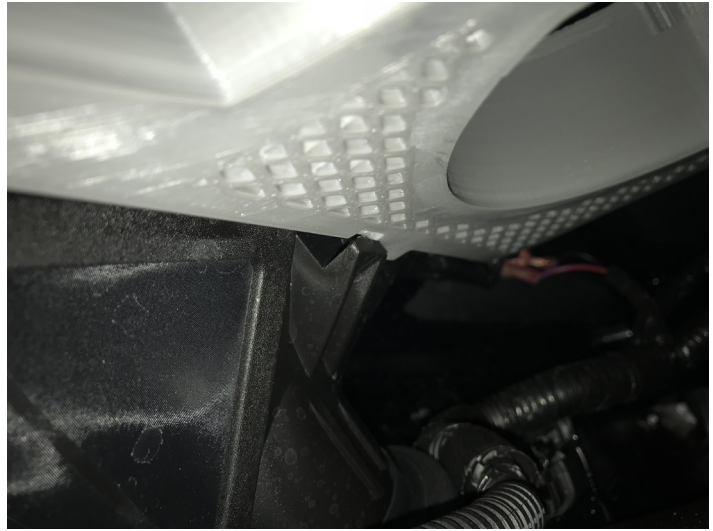
Figure 38. Relocating bracket incorrect position
