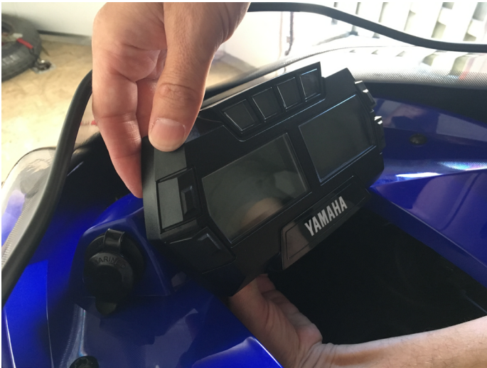
Figure 25. Instrument cluster removal
