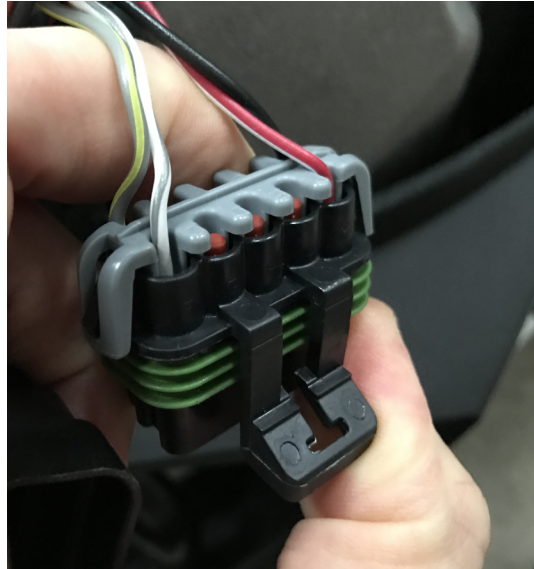
Figure 15. Diagnostic port, AEM installation
