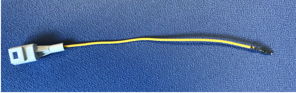
Figure 41. Optional button, harness connecting to the GAP Flasher connector
