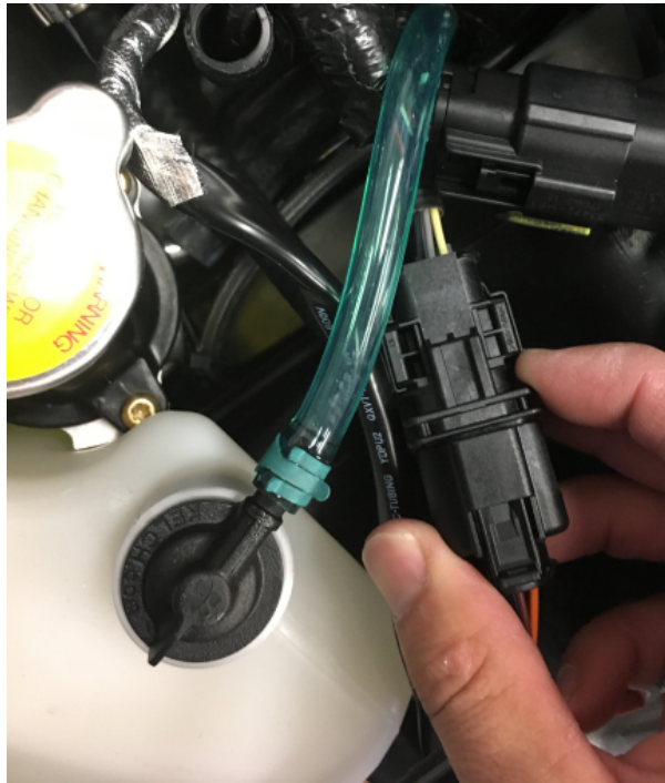
Figure 18. Connecting O2 sensor on the AEM harness
