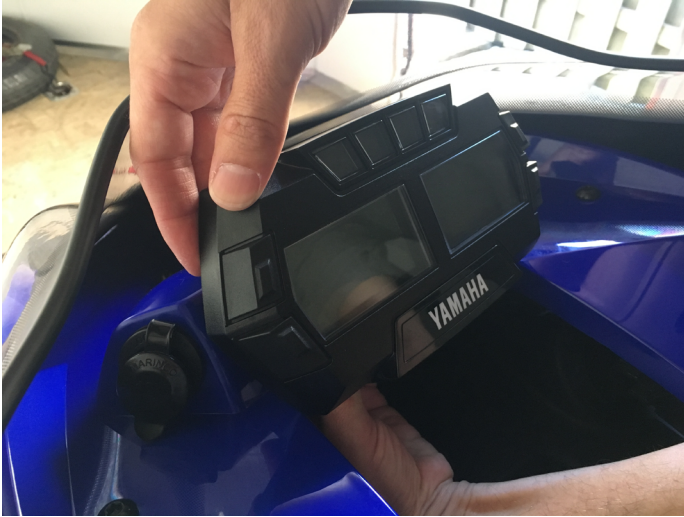
Figure 20. Instrument cluster removal
