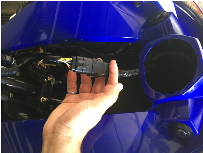
Figure 22. Connect Anti-Lag and instrument cluster harnesses
