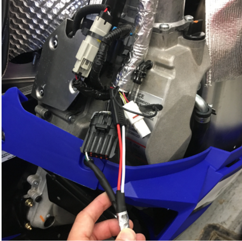
Figure 16. Connecting the AEM harness on the vehicles harness
