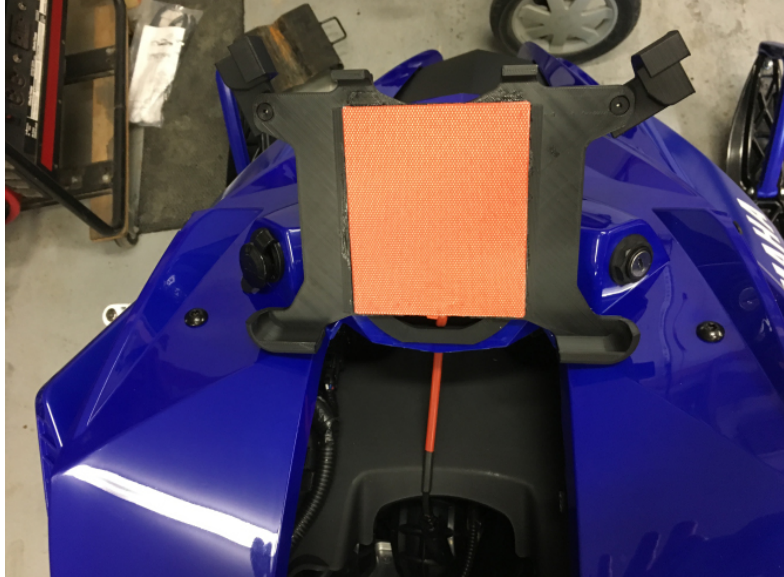
Figure 27. Installing the iPad support
