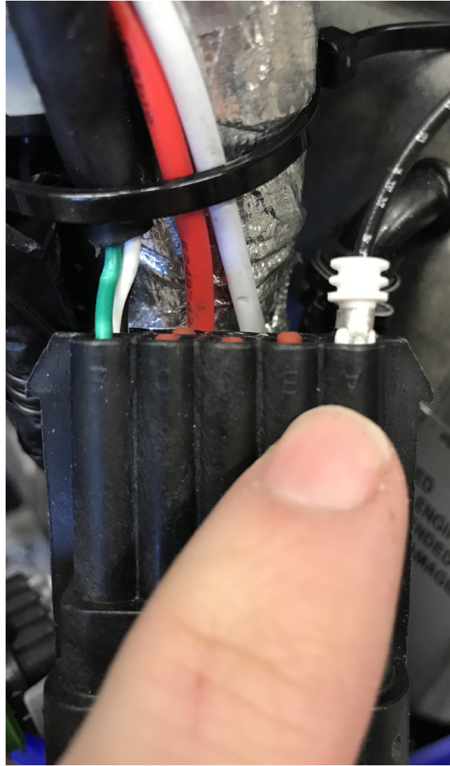
Figure 48. Optional button, black diagnostic port harness connection
