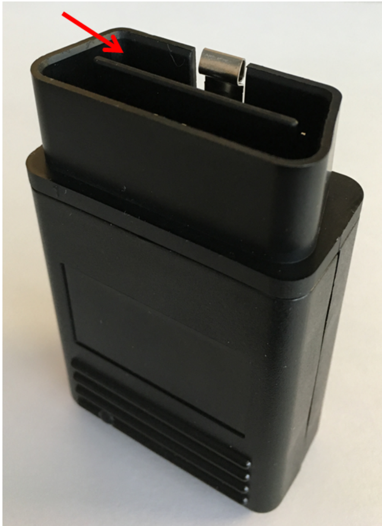
Figure 2. OBDII connector which connects the GAP Flasher to the supplied wiring harness
