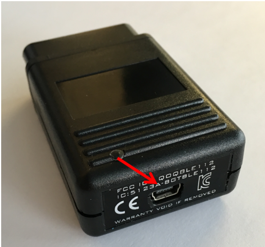
Figure 1. Micro USB socket for USB cable used to connect the GAP Flasher to a computer.
