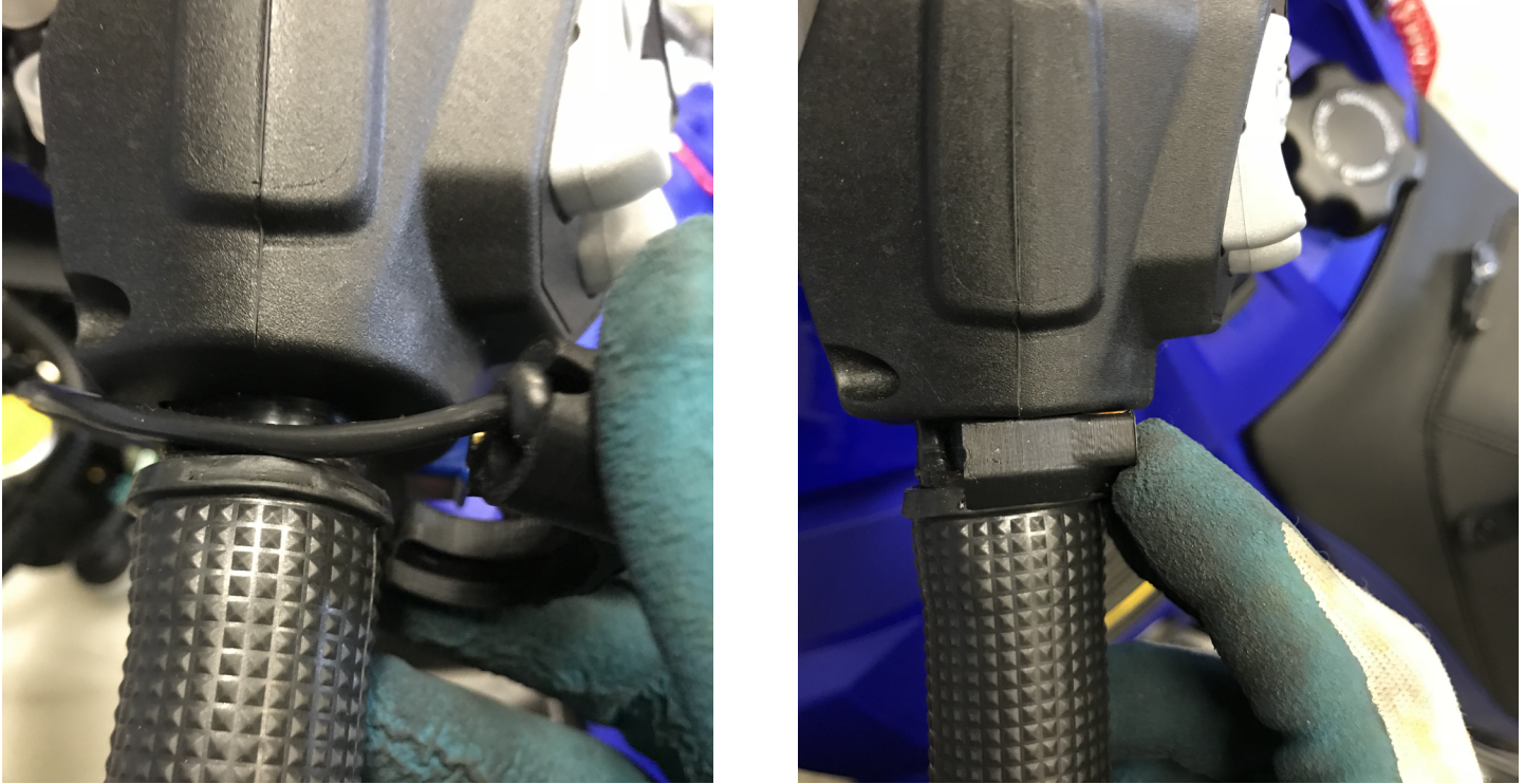
Figure 53. Button installation, button at the top (left) and bottom (right)
