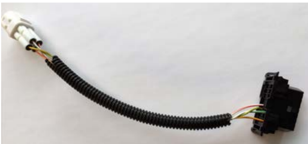
Figure 4. Wiring harness to connect on the diagnostic port of the vehicle.
