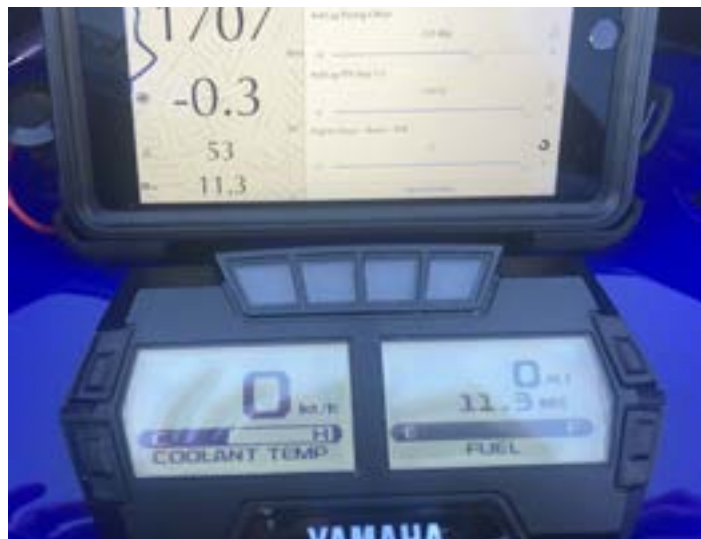
Figure 46. Optional AEM O2 broadband sensor, 11.3 AFR in this example
