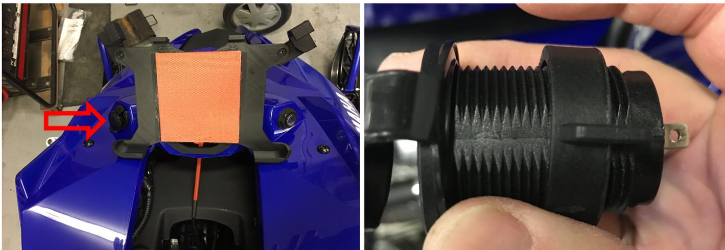
Figure 76. Prise accessoire, bague de retenue
