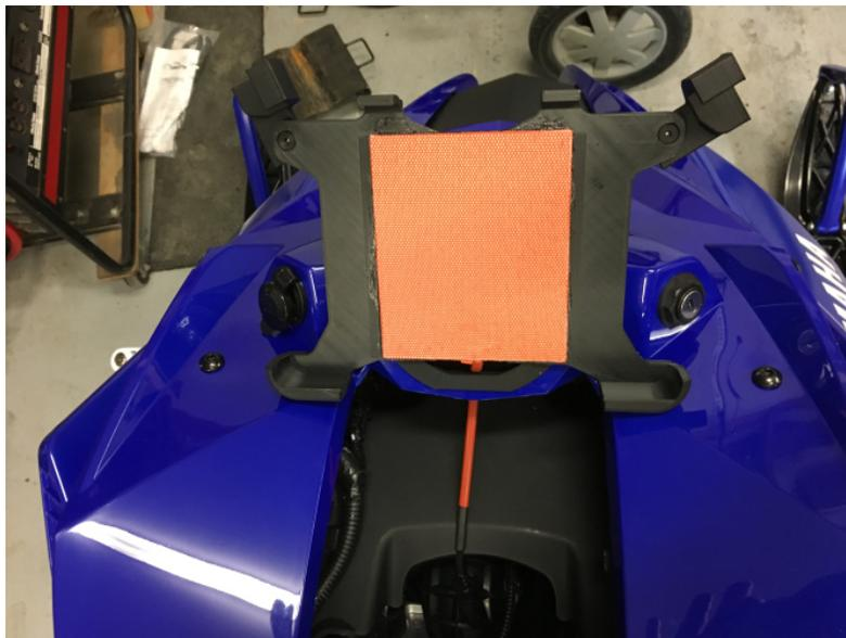
**Figure 24.** Installation du support de iPad
