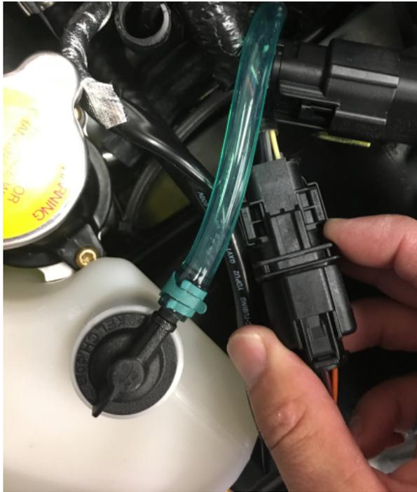
**Figure 6.** Connecting O<sub>2</sub> sensor on the AEM harness
