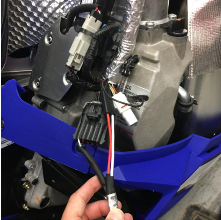
**Figure 4.** Connecting the AEM harness on the vehicles harness
