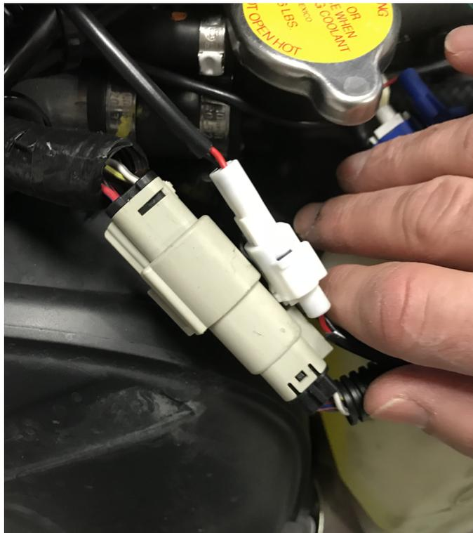
**Figure 80.** Connection at the hood junction
