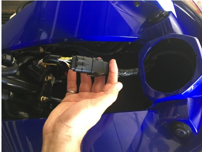
**Figure 11.** Connect Anti-Lag and instrument cluster harnesses
