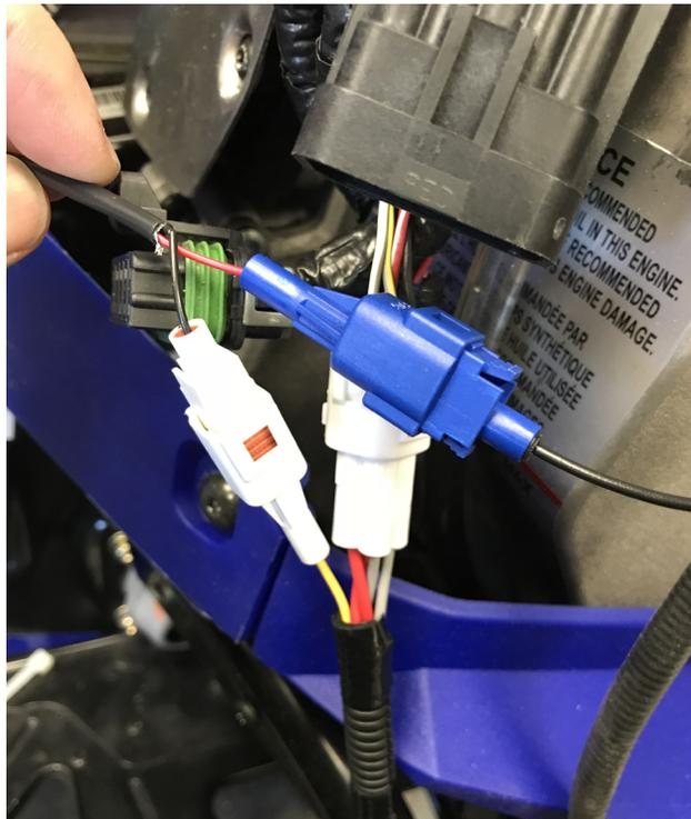
Figure 53. Cable # 3 connected to cable #1 and 2, ACC1009-U
