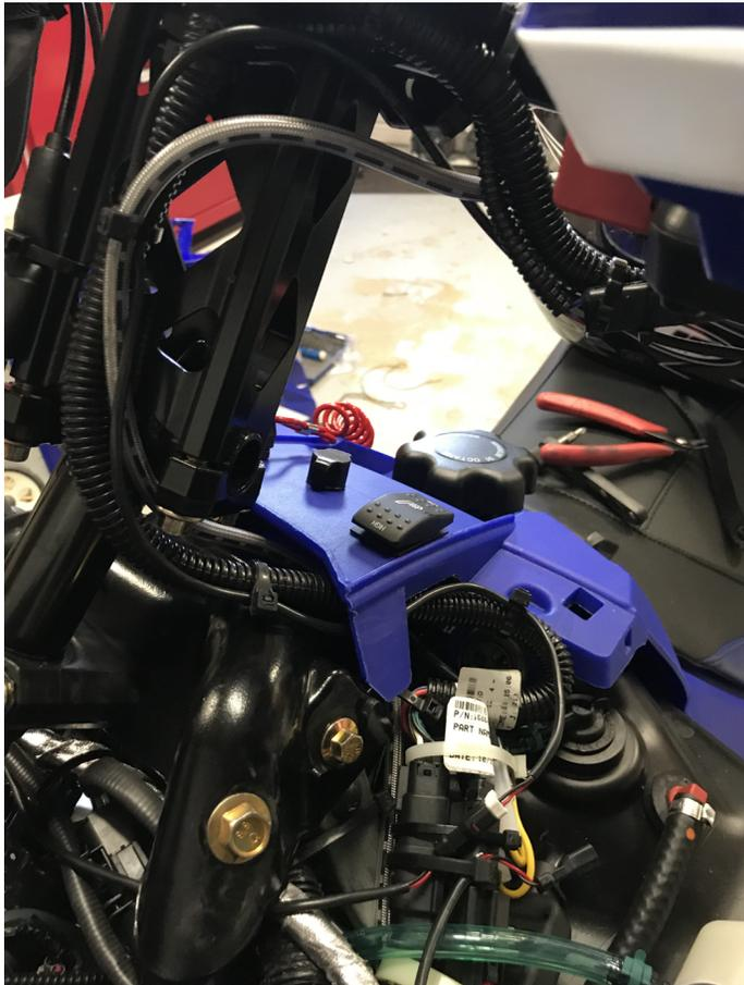
**Figure 59.** Cable # 4, routing on handlebar and steering post, ACC1009-U
