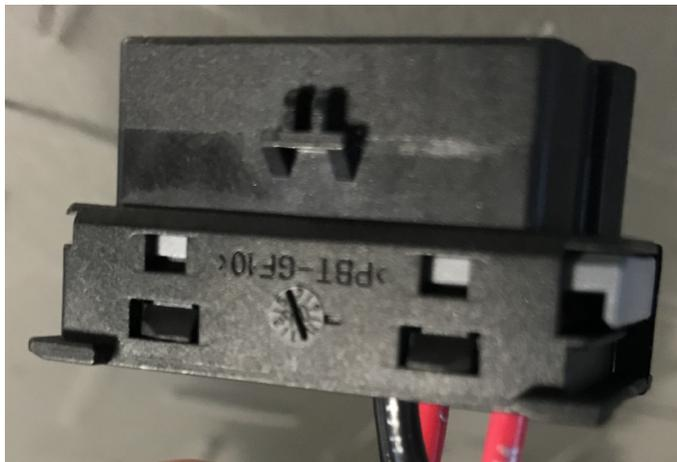
**Figure 69.** Unlock the connector, type B, ACC1007-L only
