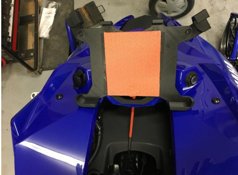
**Figure 24.** Installing the iPad support
