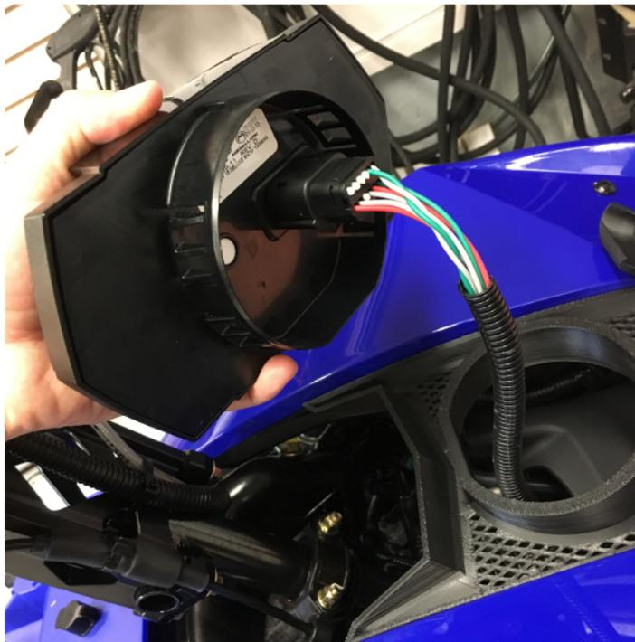
**Figure 12.** Instrument pack connection to the Anti-Lag harness
