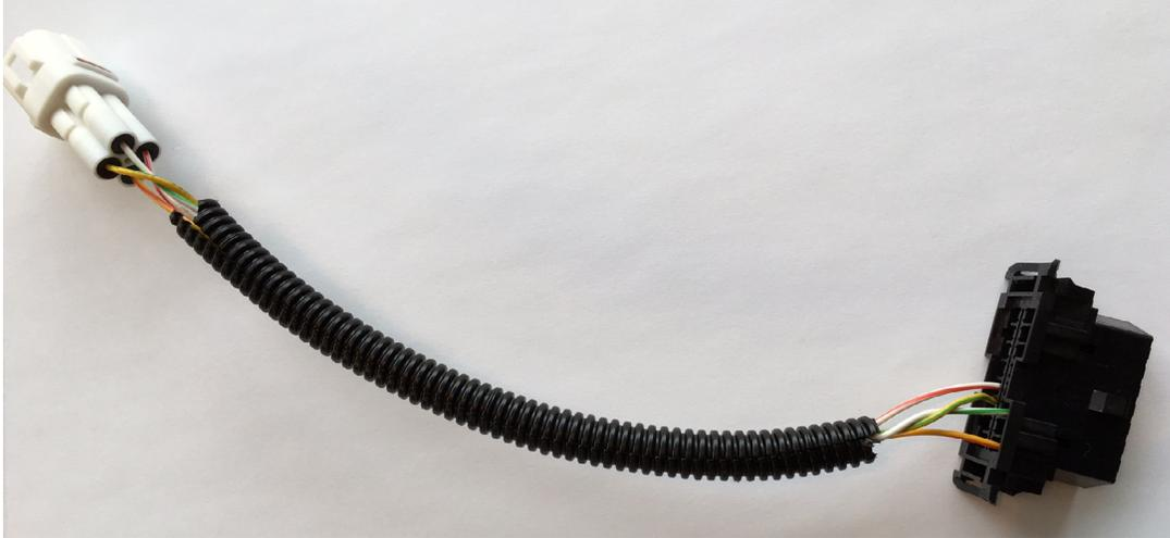
**Figure 2.** Wiring harness to connect on the diagnostic port of the vehicle.
