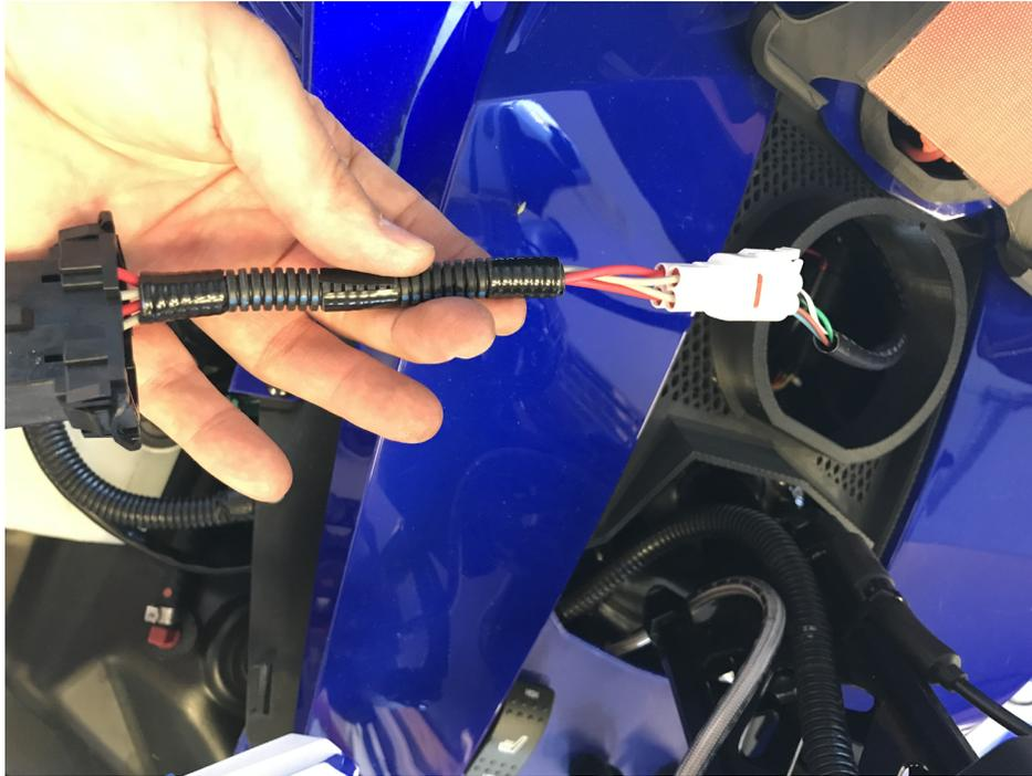
**Figure 20.** Connecting extension cable # 2 and GAP Flasher, GF1011
