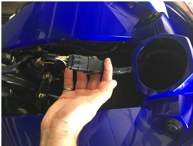
**Figure 25.** Connection of the Anti-Lag and instrument cluster harnesses
