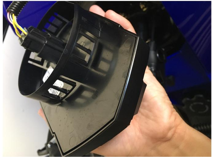
**Figure 23.** Instrument cluster locking tabs locations
