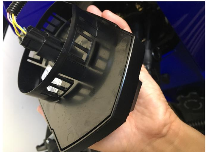
**Figure 10.** Instrument cluster locking tabs locations
