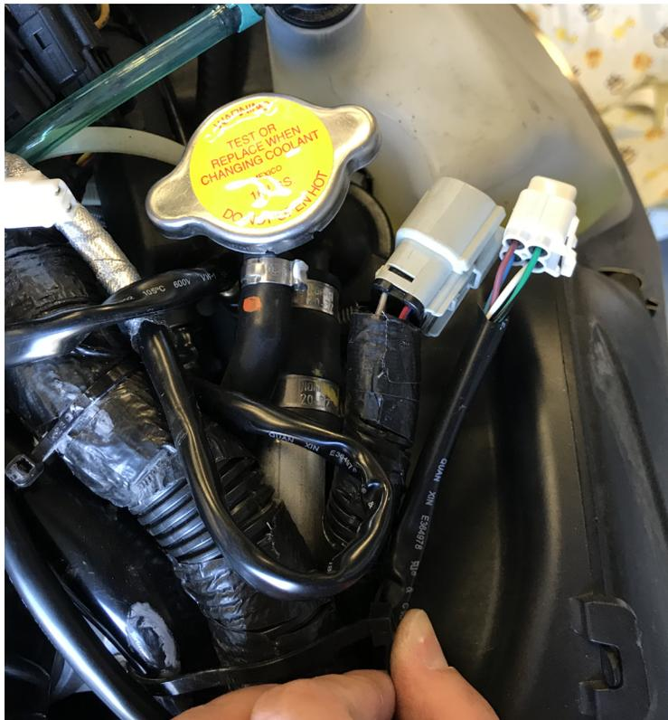
**Figure 16.** Cable # 1 routing, hood junction, GF1011
