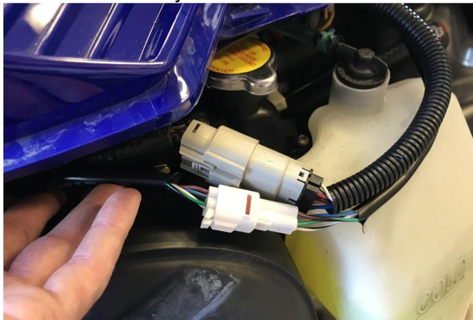
**Figure 19.** Connecting cable # 1 and # 2 at the hood junction, GF1011.
