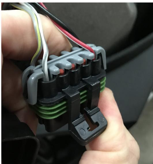
**Figure 3.** Diagnostic port, AEM installation
