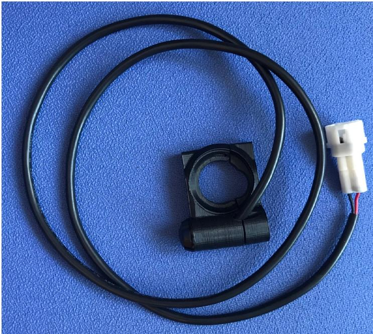
**Figure 65.** Cable # 3, optional button, ACC1007-L and ACC1008-L.
