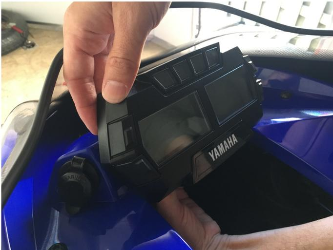
**Figure 22.** Instrument cluster removal
