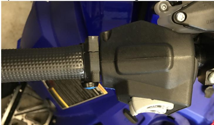
**Figure 58.** Cable # 4, button installation, back installation, ACC1009-U
