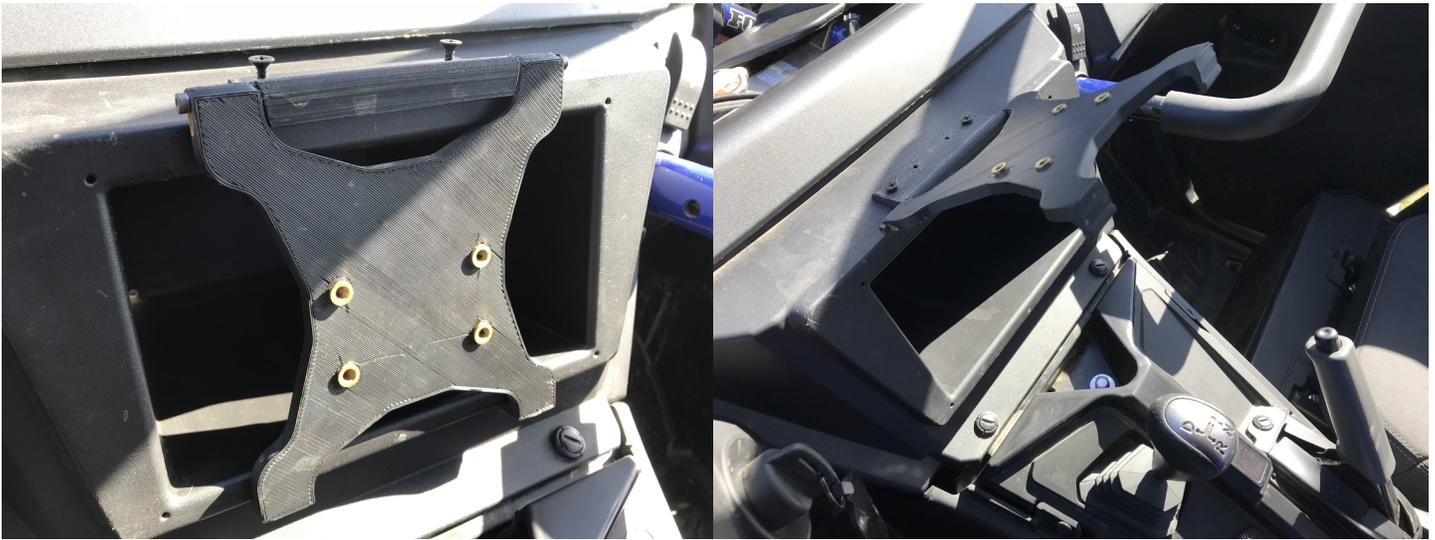
**Figure 62.** Bracket fixation with supplied screws, YXZ
