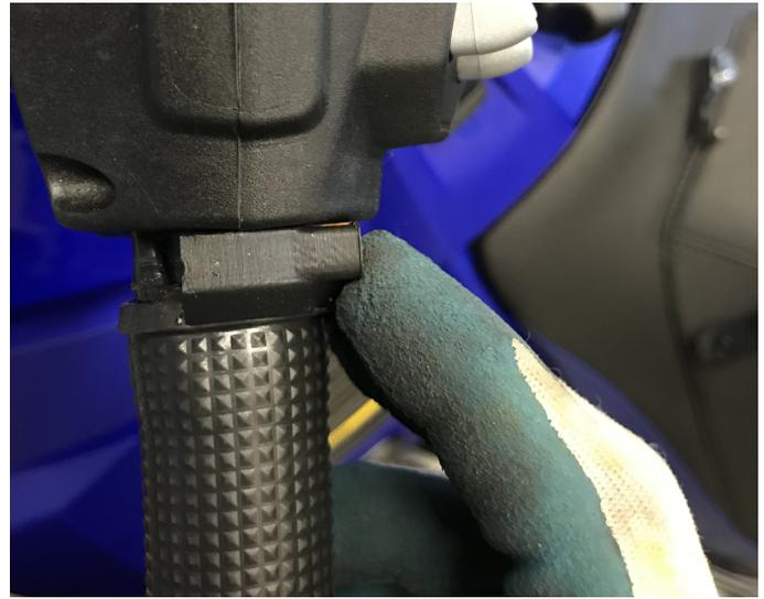
**Figure 76.** Button installation, two types, button at the top (left) or bottom (right), 998cc Arctic Cat snowmobiles
