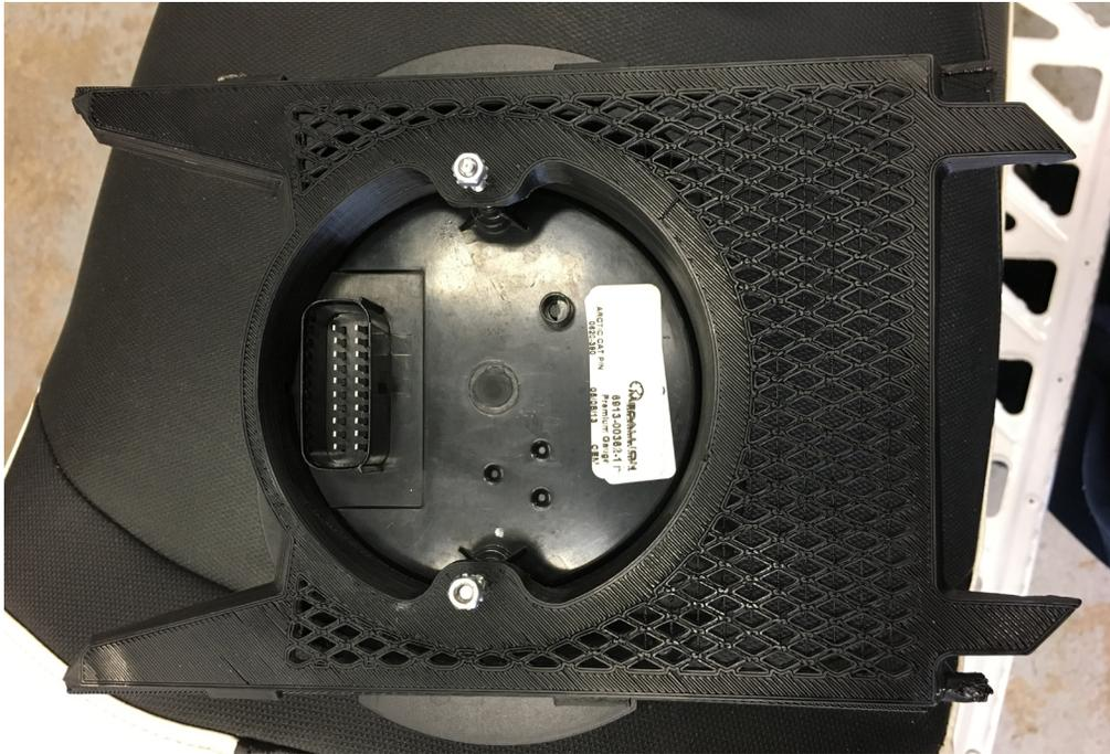
**Figure 34.** Instrument cluster installed on relocating bracket, 1100cc Arctic Cat snowmobiles
