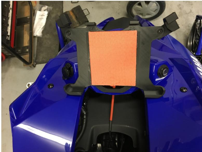
**Figure 6.** Installing the iPad support 998cc Turbo snowmobiles
