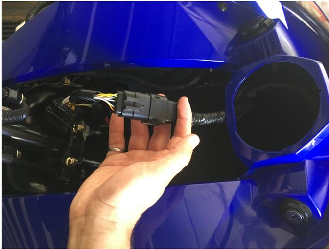
**Figure 7.** Connect CoPiTrail and instrument cluster harnesses 998cc Turbo snowmobiles
