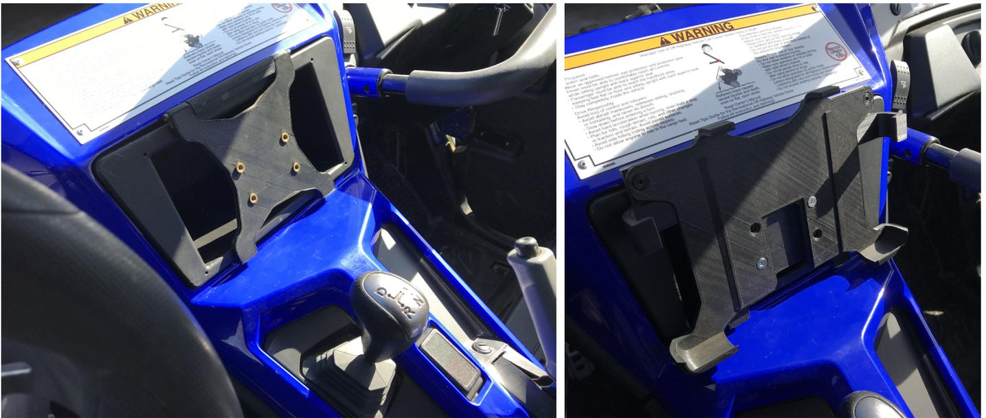
**Figure 63.** iPad support installation with supplied screws, YXZ
