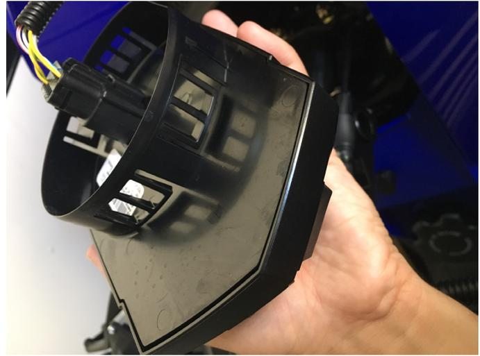
**Figure 4.** Instrument cluster locking tabs locations 998cc Turbo snowmobiles
