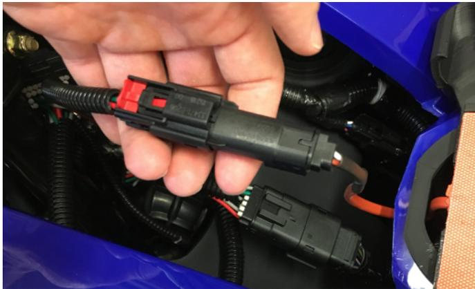
**Figure 8.** Connect the heating pad to the CoPiTrail harness 998cc Turbo snowmobiles
