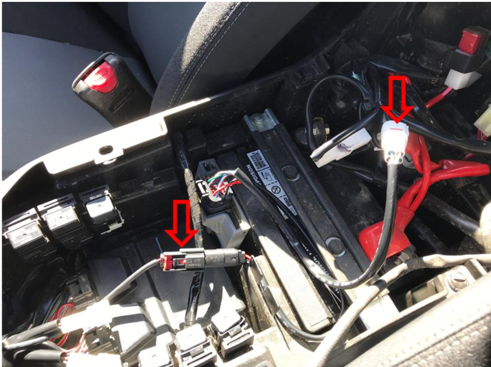
**Figure 58.** Connections to CoPiTrail main harness, YXZ
