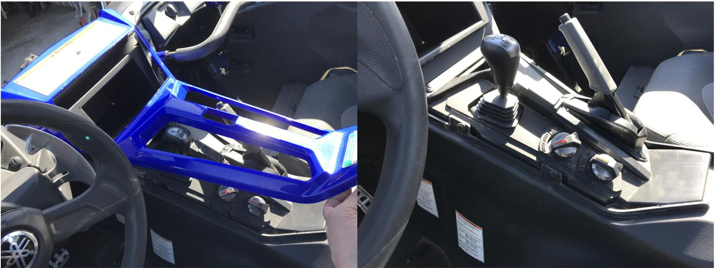
**Figure 49.** Centre console cover lift and removal, YXZ
