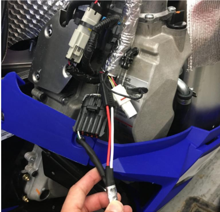
**Figure 66.** Connecting the AEM harness, 998cc Arctic Cat snowmobiles
