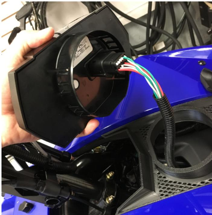
**Figure 21.** Instrument pack connection to the CoPiTrail Harness, 998cc Turbo snowmobiles
