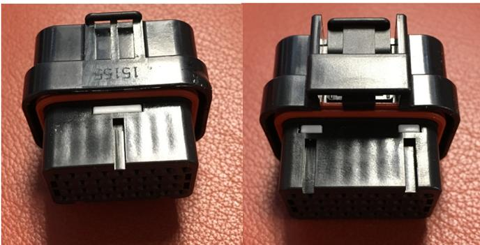
**Figure 31.** Locked connector
