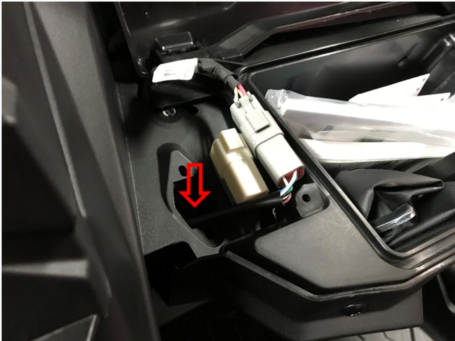
**Figure 43.** CoPiTrail harness connected to the diagnostic port, Can Am Maverick
