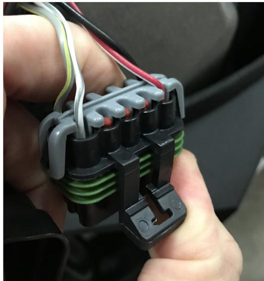
**Figure 64.** Diagnostic port, AEM installation, 998cc Arctic Cat snowmobiles
