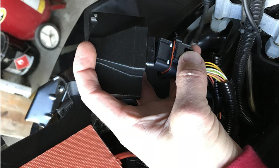
**Figure 26.** Connect the CoPiTrail module, 1100cc Arctic Cat snowmobiles
