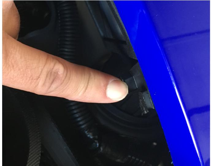
**Figure 12.** Instrument panel tabs locations, 998cc Turbo snowmobiles
