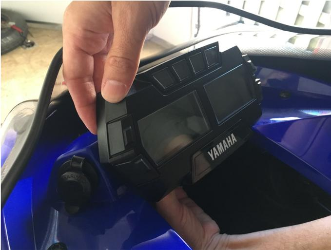
**Figure 3.** Instrument cluster removal 998cc Turbo snowmobiles
