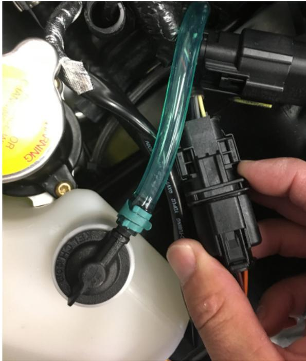
**Figure 68.** Connecting the sensor on AEM module, 998cc Arctic Cat snowmobiles
