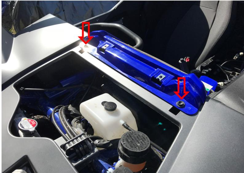
**Figure 47.** Centre console cover screw removal, YXZ
