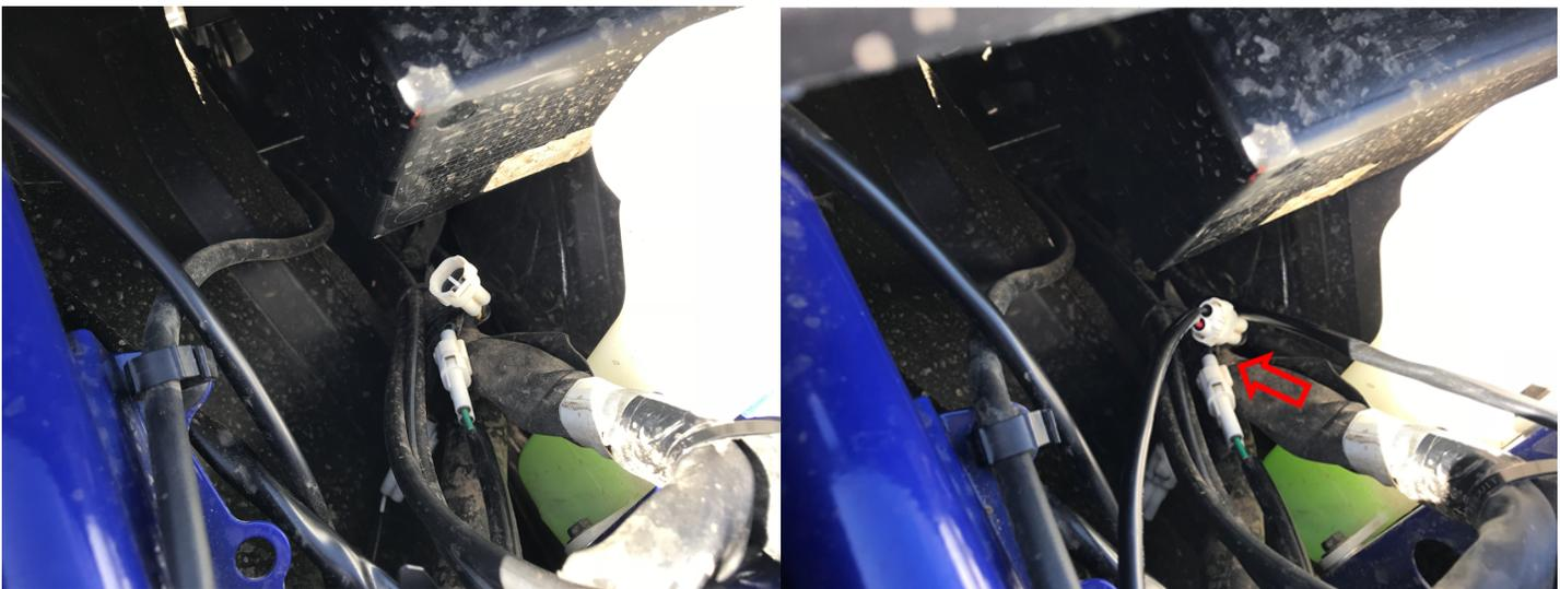
Figure 54. Ignition cable connection at the accessory connector, YXZ
