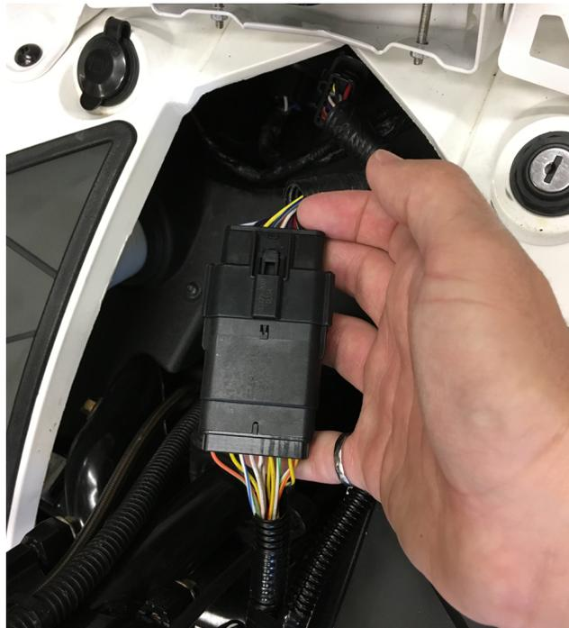
**Figure 25.** Connecting the CoPiTrail harness to the instrument cluster harness, 1100cc Arctic Cat snowmobiles
