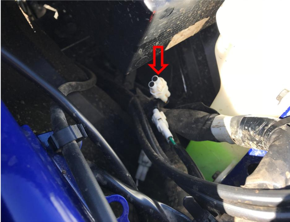
Figure 53. Accessory connector location, YXZ
