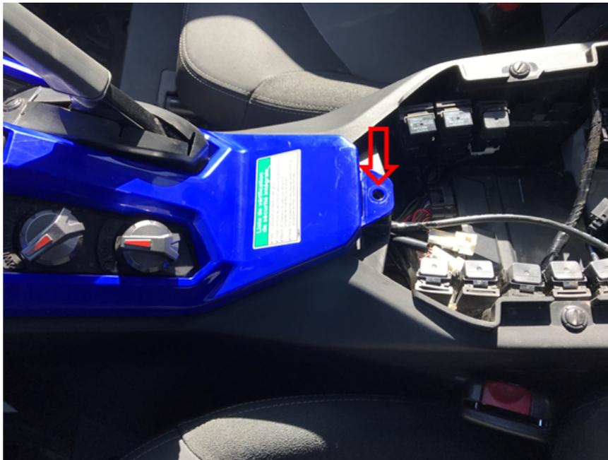
**Figure 48.** Centre console cover clip removal, YXZ
