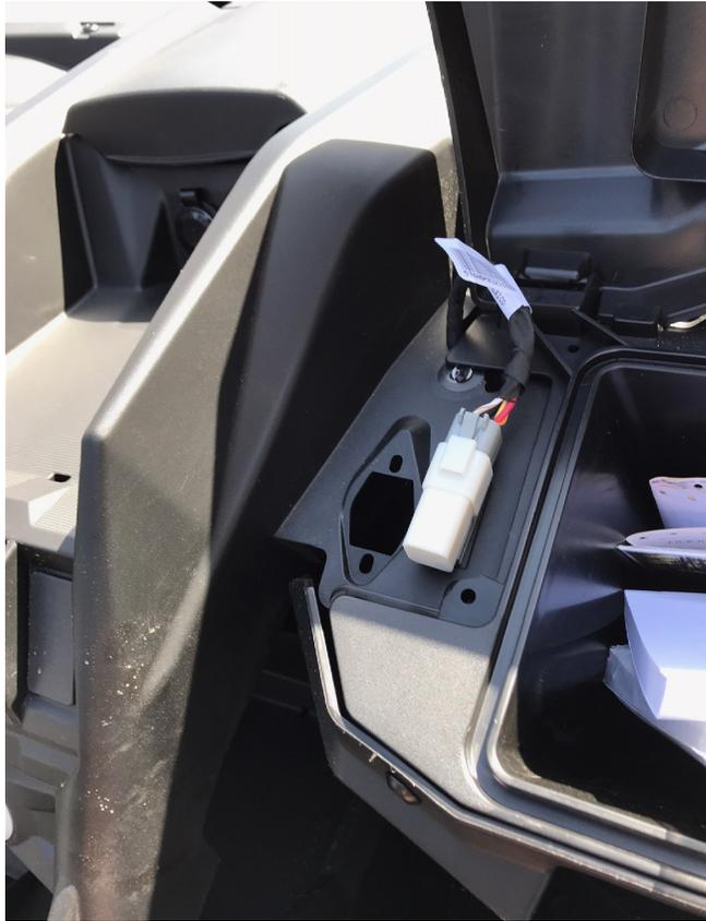
**Figure 42.** Diagnostic connector, Can Am Maverick
