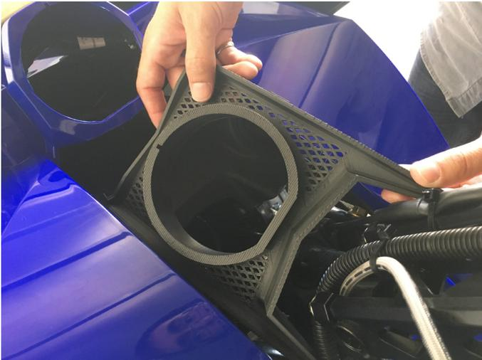
**Figure 13.** Relocating bracket initial steps, 1, 998cc Turbo snowmobiles
