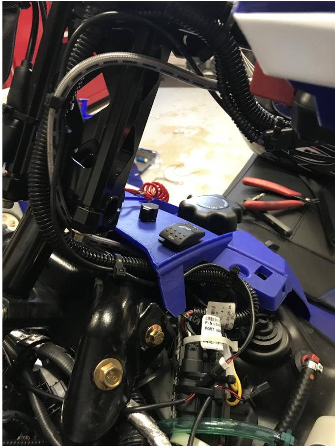
**Figure 78.** Routing on handlebar, 998cc Arctic Cat snowmobiles
