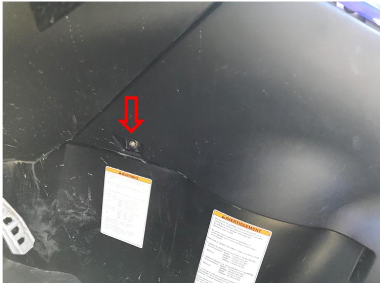
**Figure 50.** Side console screw removal, YXZ
