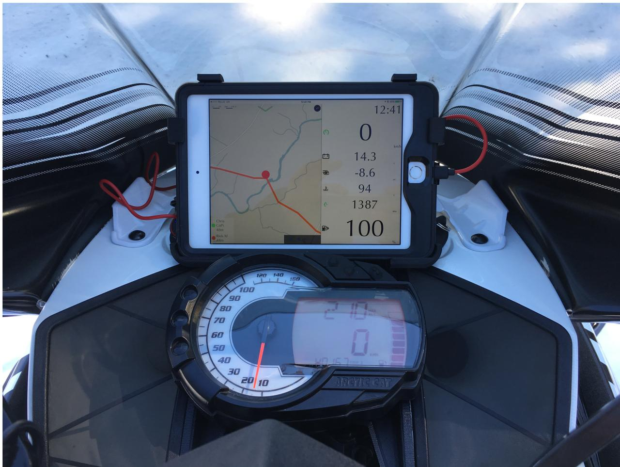
**Figure 23.** CoPiTrail installed overview 1100cc Arctic Cat snowmobiles
