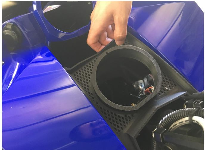
**Figure 14.** Relocating bracket initial steps, 2, 998cc Turbo snowmobiles
