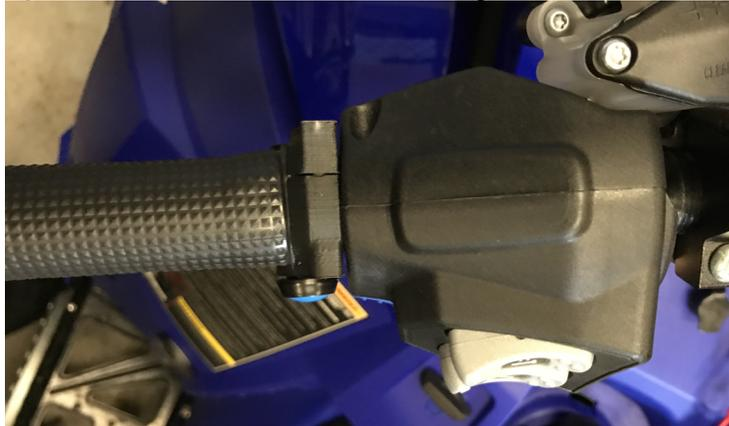
**Figure 77.** Button installation, back installation, 998cc Arctic Cat snowmobiles
