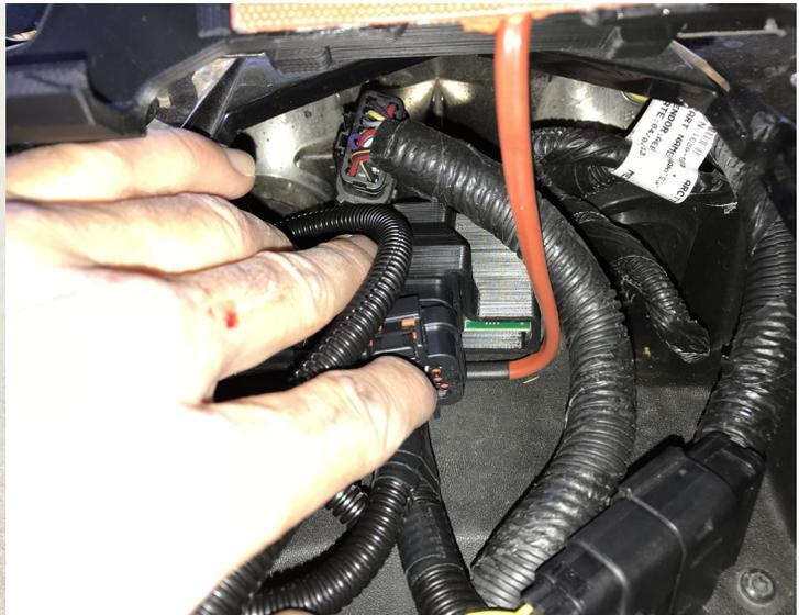
**Figure 27.** Fix the CoPiTrail module, 1100cc Arctic Cat snowmobiles
