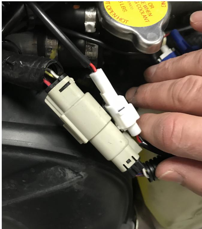
**Figure 79.** Connection at hood connector, 998cc Arctic Cat snowmobiles
