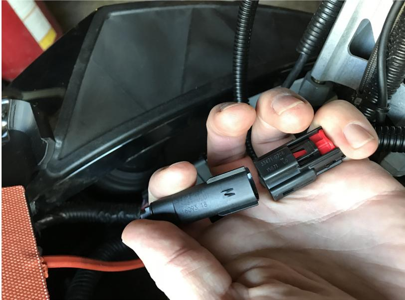
**Figure 30.** Heating pad connection, 1100cc Arctic Cat snowmobiles
