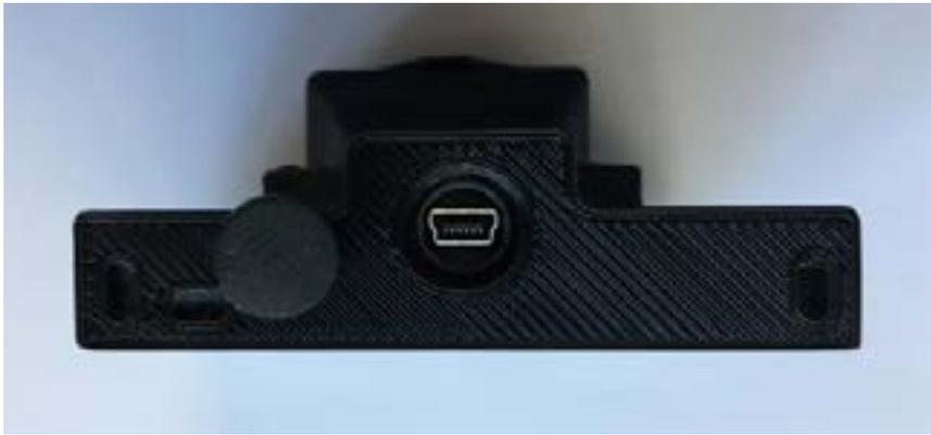
**Figure 1.** Micro USB socket for USB cable used to connect the CoPiTrail to a computer. **Remove cover for access**
