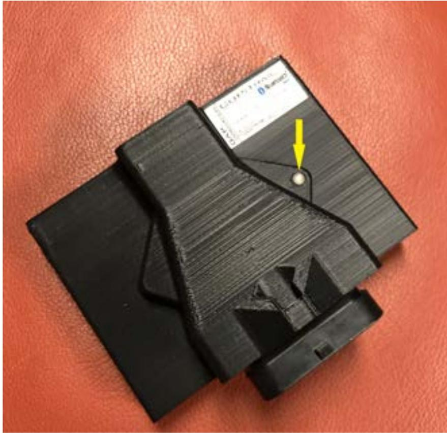
**Figure 4.** Status LED used for diagnostic purposes.
